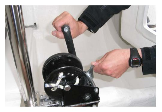
Keel should be angeled about 5-10 degrees to the aft in its working position. If the keel hoist line is loose it probably means you droped it to far forward.
