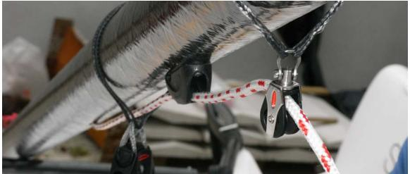
Attach this rope to the thiner one (tie together the two lines – the knot is hidden in the boom) which you lead out trough the block at the end of the boom. You use 1:2 purchase when attaching outhaul line to the mainsail as shown on the photo:
