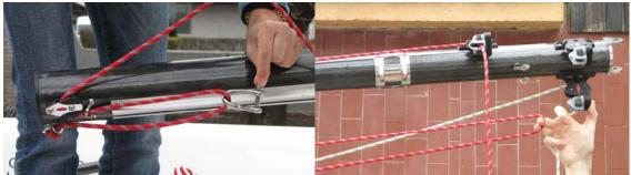
Then the jib hallyard. Make shure to make a knot connecting both ends to prevent the hallyard from falling out of the top furler when hoisting.
