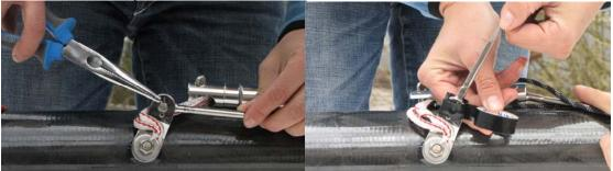
On the bottom part of the shrouds attach turnbuckles to the chainplates as shown on the next photo. After you insert the safety pin aplly generous ammount of electric tape to prevent the spinnaker sheets catching in the pin. Make shure that the turnbuckles are maximaly unwinded to allow raising of the mast:
