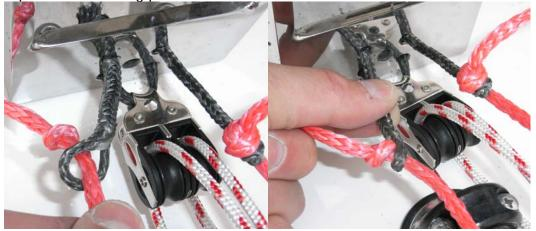
Don't cut the cascade lines before the system streches. When you are satisfied with the mobility of the boom (it has to move at least 10deg up and down from horizontal position) you can cut the lines to right length.
