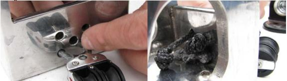
The system suplied is 1:12 purchase. In stronger wind (20-25+ knots) this system allowes significant force to be put to the boom so be advised that you can damage the boom if you overtension the vang in this conditions. The use of composite shackles is explained in following photos:
