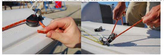
Make shure that ratchet is turned the right way (it should block the sheet towards the gennaker when under load).
