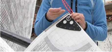
When hoisting make shure that bolt rope doesn't slide out of the groove. In that case lower the main until bolt rope is again fully inside the groove and resume hoisting. Make shure you hoist tha main all the way to the top (beforehand make shure vang, main sheet and cunningham are released).
