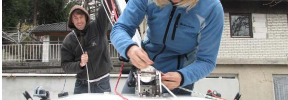
You raise the mast to its final position. Person from the back of the boat is raising the mast by hand and by walking towards the front, the other is collecting the asymetric spinnaker hallyard which is in the process replacing the forestay.
