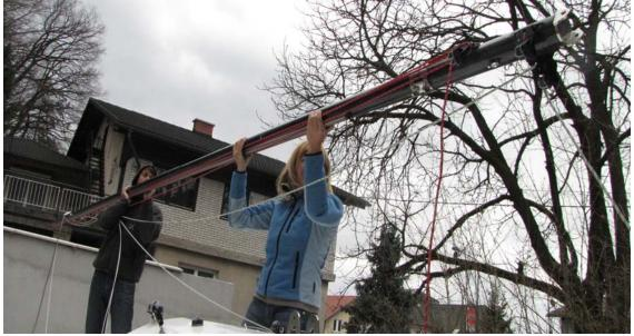
The person at the back uses his shoulder to support the weight of the mast and the person at the mast step alignes the mast with the mast foot. In order to help aligning the holes the person supporting the mast gently moves the mast few centimeters left and right. Then you insert the bolt into the mast step and secure it with the safety pin:
