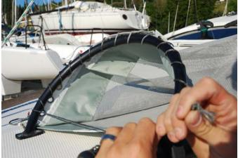
Then take the end of gennaker hallyard, run it trough the block on the left side of the cockpit (next to the gennaker sheet block) and trough the bag. Attach the sheet blocks: 40mm normal in the back and 40mm smart ratchet in the front
