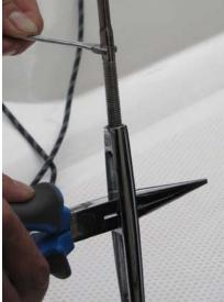
When raised top of the mast should look like something like that (you can find two mistakes on photo below: only one shroud is secured with electric tape and loop for forestay is not nicley aligned):
