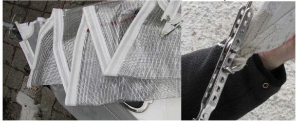
Then attach both ends of the forestay to the top of the jib and zip up the jib halyard and the forestay. Hoist the jib and make a knot at the bottom of the jib hallyard that will create a loop for jib cunningham:
