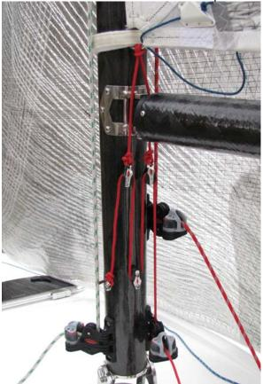
Top is attached to the hallyard with shackle due to 2:1 halyard system:
