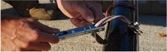
After you insert the pin and secure it with the safety splice. When you finish protect it with the electric tape.
