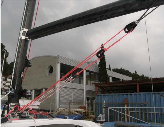
Make shure that the loop around the boom that distributes the force of the vang, isn't tangled and runs smoothly:
