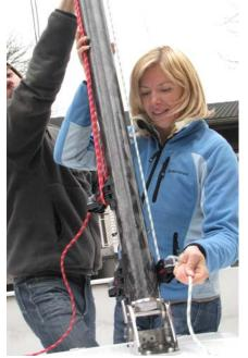
Next step is attaching the forestay. You attach furler with the drum, to forestay chainplate. Tension the asymetric spinnaker hallyard as much as needed to insert the forestay into desired hole. 5<sup>th</sup> from the top is a good start before you start playing with the trim...
